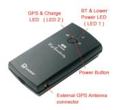
The Bluetooth GPS has two LED lights, each having two colors. One is Bluetooth & low power status LED, named LED 1 and the other is GPS & Charge status LED, named LED 2. The status table of the LEDs is given by:
