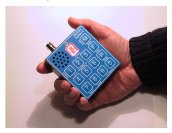
The VK3YNG Foxhunt Sniffer is a specially designed synthesised VHF direction finding receiver covering 120MHz and 144MHz bands.
