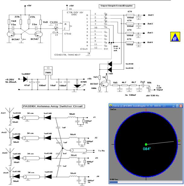
Homebuild VHF/UHF DSP Direction Finder connected to the soundcard off the PC.
