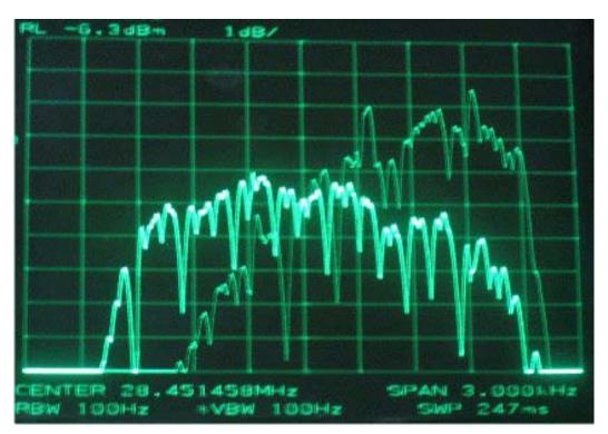
The above picture shows the effect of switching the processor on. The radio has been fed with a slow audio sweep, and the Spectrum analyser scale has
