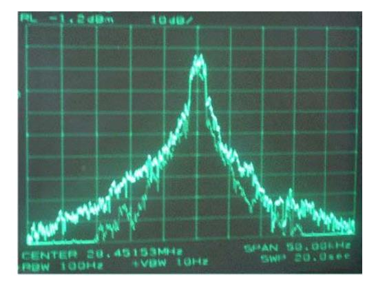
The bright trace shows the radio with maximum mic gain and processing and full ALC operation (worst case). The dim trace shows low mic gain with no processing, just before the onset of ALC. The top graticule line represents 100W CW power, the span is 50KHz so each division represents 5KHz. Note that the difference in peak levels of the wanted signal are only a few dB's but the unwanted skirts are quite a bit higher.
