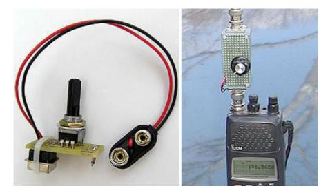
Marvin Johnston also offers the attenuator circuit board mounted inside the boom of a WB2HOL-style measuring-tape beam. Actually, the circuit is inside a plastic pass-through electrical box (with waterproof gasket) that is incorporated into the PVC pipe boom. While holding the mast of the beam, you can adjust the attenuator with the thumb of the same hand. Kits are now available directly from Marvin.
