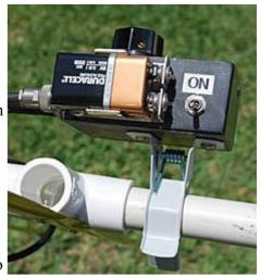
3. When working properly, the offset frequency signal should decrease smoothly as the control knob is turned counterclockwise, with maximum attenuation of over 100 dB achieved at the counterclockwise
