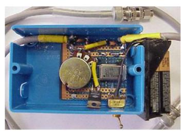
At left: The photo by Wayne Yoshida KH6WZ shows how he built his unit into a plastic electrical box, which he found for less than a dollar at a hardware store. SuperStrong Adhesive from 3M (not shown in the photo) holds the coax in place and provides strain relief. The
