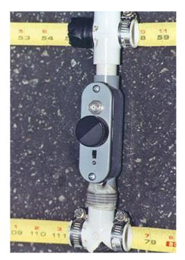
**A complete offset attenuator with enclosure and connectors,** ready to use, is available from this model by Arrow Antennas, shown below. It uses a miniature coin-cell lithium battery. A product review is in my Winter 2006 **Homing In** column for *CQ-VHF Magazine*.
