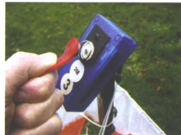
PHOTO 4: 'Punching' at one of the control boxes. The 45° angle makes this easy and at the same time allows rainwater to drain away easily.
