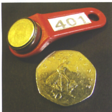
PHOTO 1: The iButton mounted in a key fob with a 50p piece for scale.
